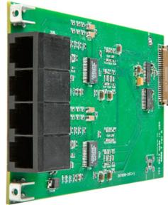
QUAD-TEL is a 4 channel (2 inputs, 2 outputs) modular telephone interface card for use with Ivie MAP series devices. The QUAD-TEL allows a MAP system device to connect directly to standard analog telephone lines. Each channel includes caller-ID decoding, ring detection/validation, DTMF decoding, and call progress tone decoding. Each channel includes a second connector in parallel for pass through to a telephone.
