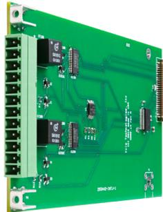
The QUAD-AES OUT is a modular digital output card for use with Ivie MAP series devices. Each QUAD-AES OUT provides 2 stereo paired channels of either AES3 or SPDIF output on euro-block connectors. AES3 (balanced and unbalanced) and SPDIF formats are continuously output on both stereo pairs. Selection of format is made by connection, and No programming is necessary.
