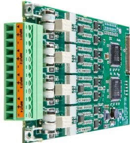
The QUAD-AEC is a 4 channel modular analog input card for use with Ivie MAP series devices. Each Quad-AEC provides 4 channels of balanced mic/line audio input with Automatic Echo Cancellation (AEC). Inputs are electrically balanced and provided on euro-block connectors.
